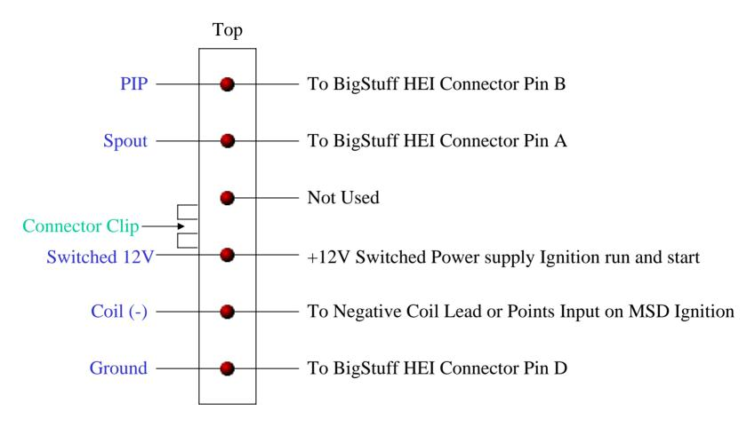
Note: The BigStuff3 "Points" wire & Pin C in the HEI connector are not used with the Ford TFI Ignition!
